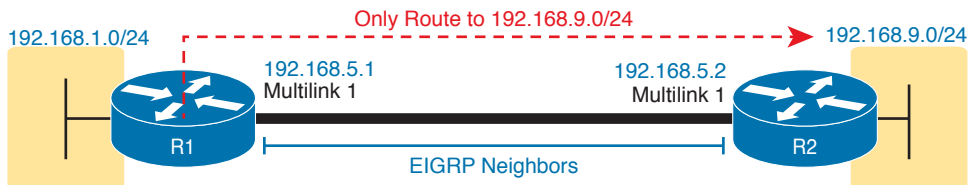
Figure 13-19 Layer 3 Concept Created by Multilink Interface
