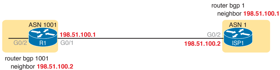
Figure 12-11 Using Link Addresses for BGP Peering in a Single-Homed Design
