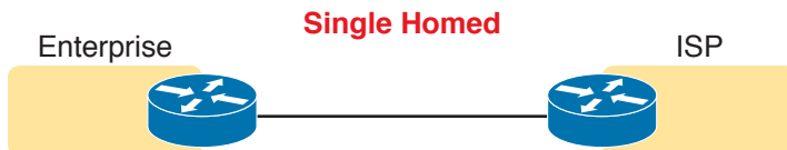
Figure 12-4 Single-Homed Design: Single Link, One Home (ISP)
