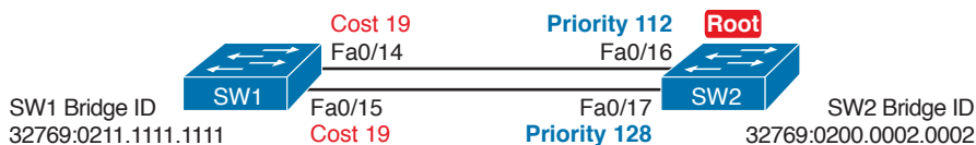
Figure 4-2 Topology Required for the Last Two Tiebreakers for Root Port
