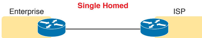
Figure 12-4 Single-Homed Design: Single Link, One Home (ISP)
