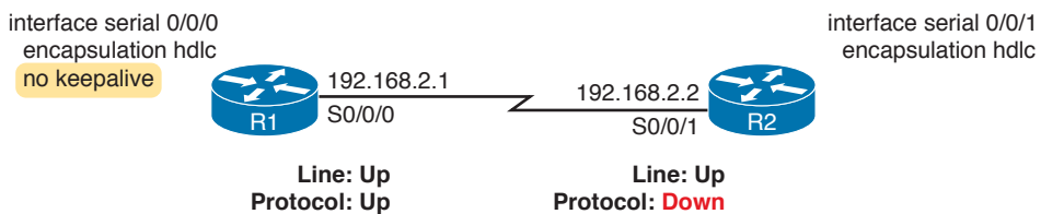
Figure 13-23 Results when Using HDLC with a Keepalive Mismatch
